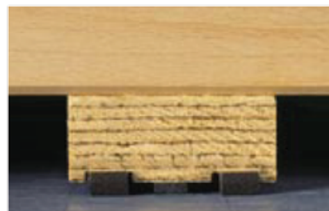
Rubber strips with maximum load (note that the outer strips are never squeezed to destruction level thanks to the centre strip and their recessment).
